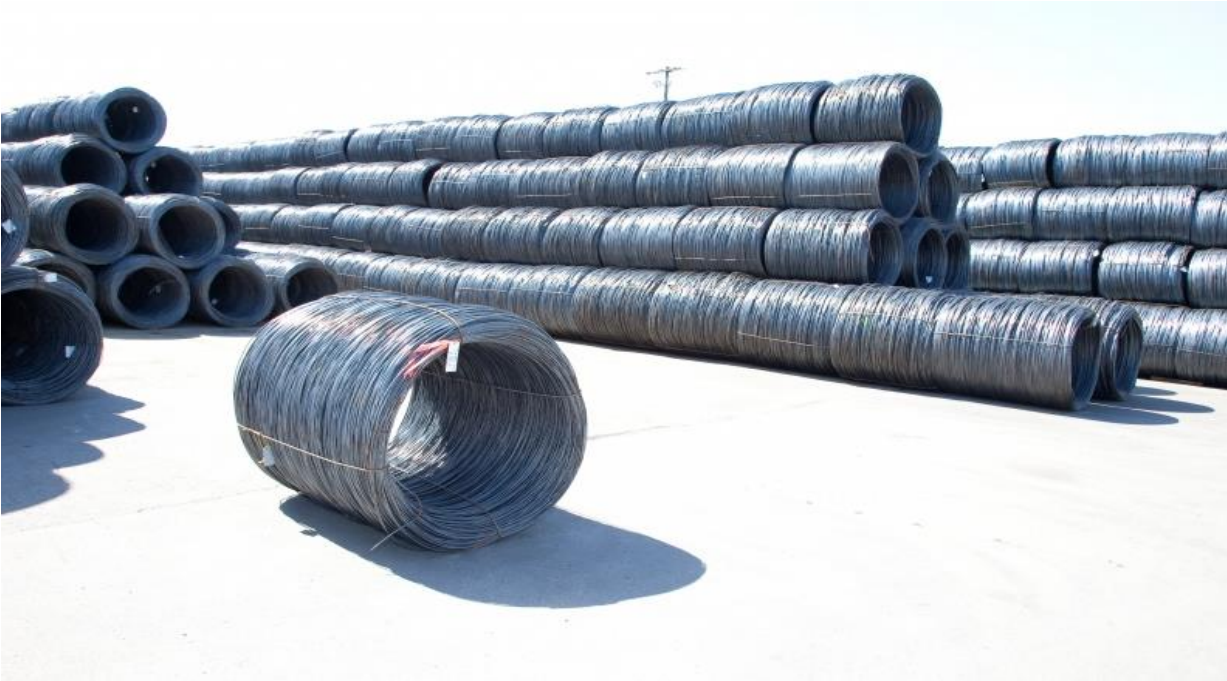
Figure 10.1-2: A typical rod yard where coils are temporarily stored
