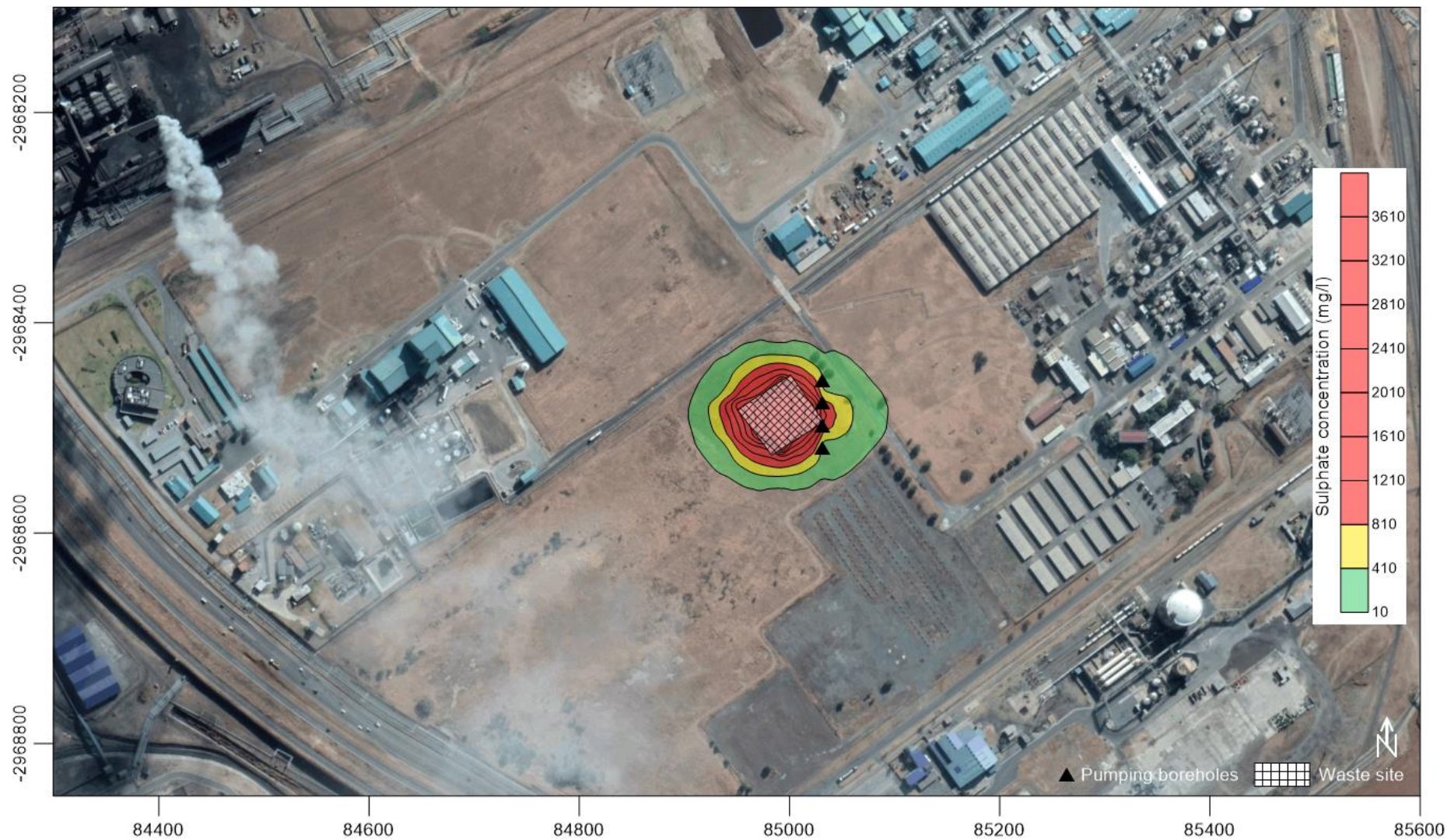
Figure 31: 40-year simulation of contamination plume with clay capping and pumping as a remediation techniques
