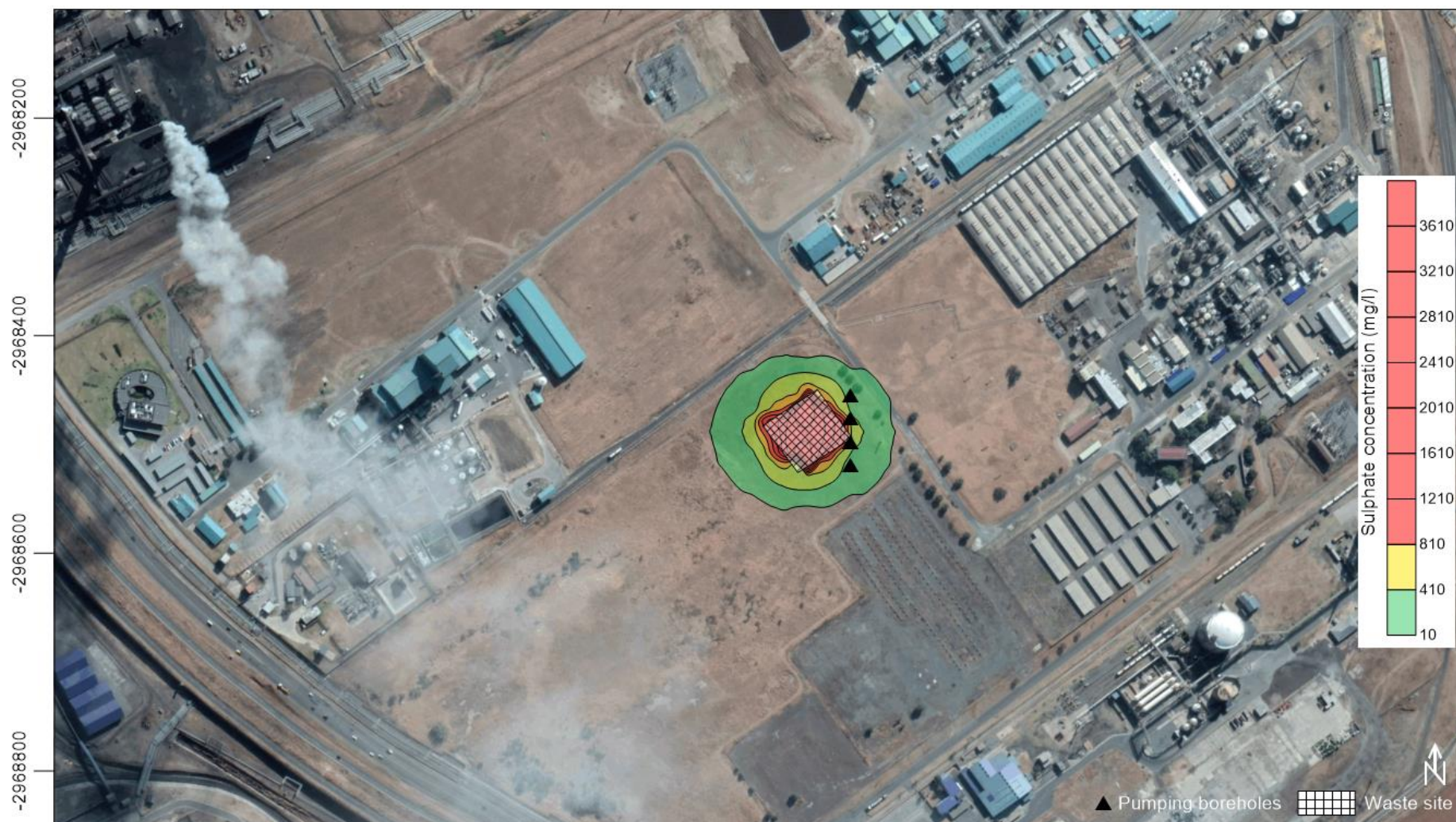
Figure 30: 40-year simulation of contamination plume with geomembrane capping and pumping as a remediation techniques
