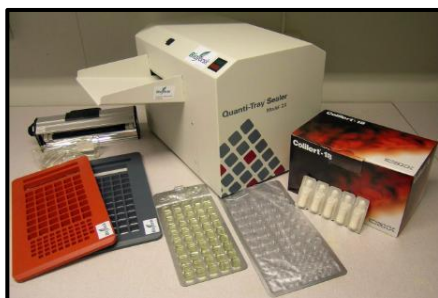
Figure 3-2: (a) Colilert-18 ® reagents and consumables used for enumeration of E.coli and total coliforms. (b) Yellow wells indicating the presence of total coliforms, fluorescent wells indicating the presence of E.coli . (Paruch, 2010)
