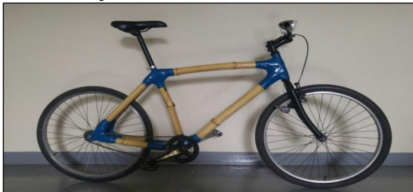
Figure 7: Manufactured bamboo bicycle [22].
