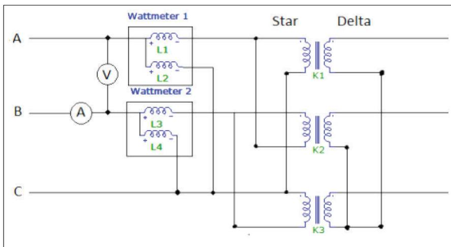
Fig. 2: Connection diagram for the open-circuit test.
