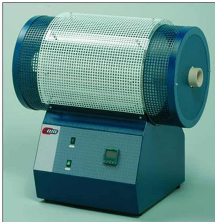
Figure 3.2 Tube furnace used in the thermal pre-treatment CTP samples
