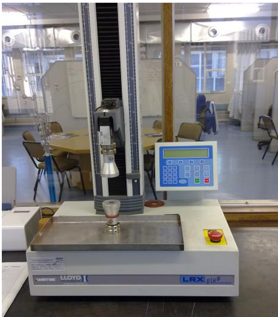
Figure 3.3 Tensile test machine used in pressing CTP pellets
