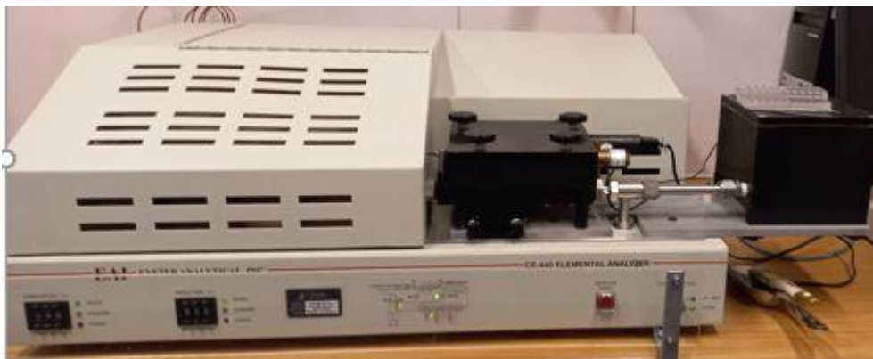
Figure 3.4: The CE-440 elemental analyser
