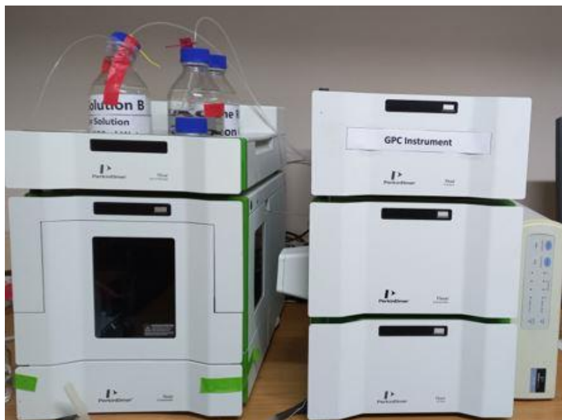
Figure 3.8: The PerkinElmer Flexar system used for GPC analysis
