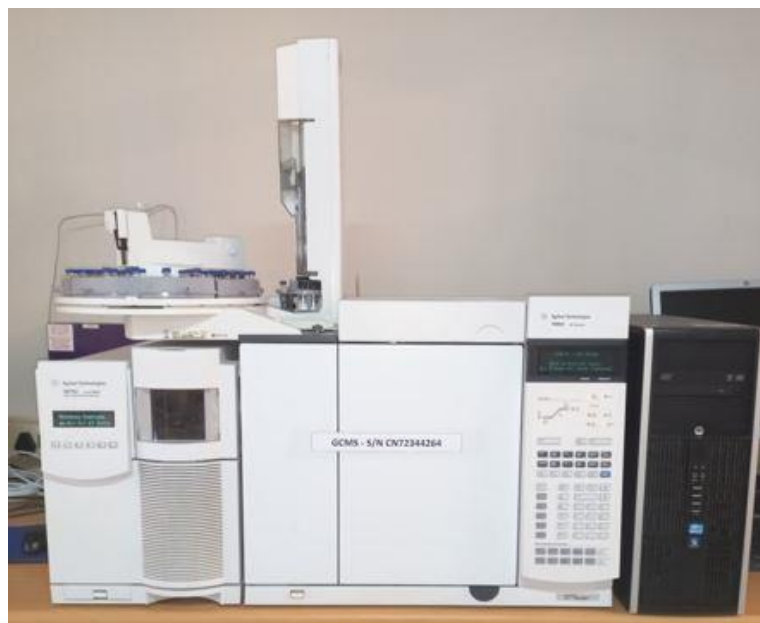
Figure 3.9: The 7890 Agilent GC system used for GCMS analysis
