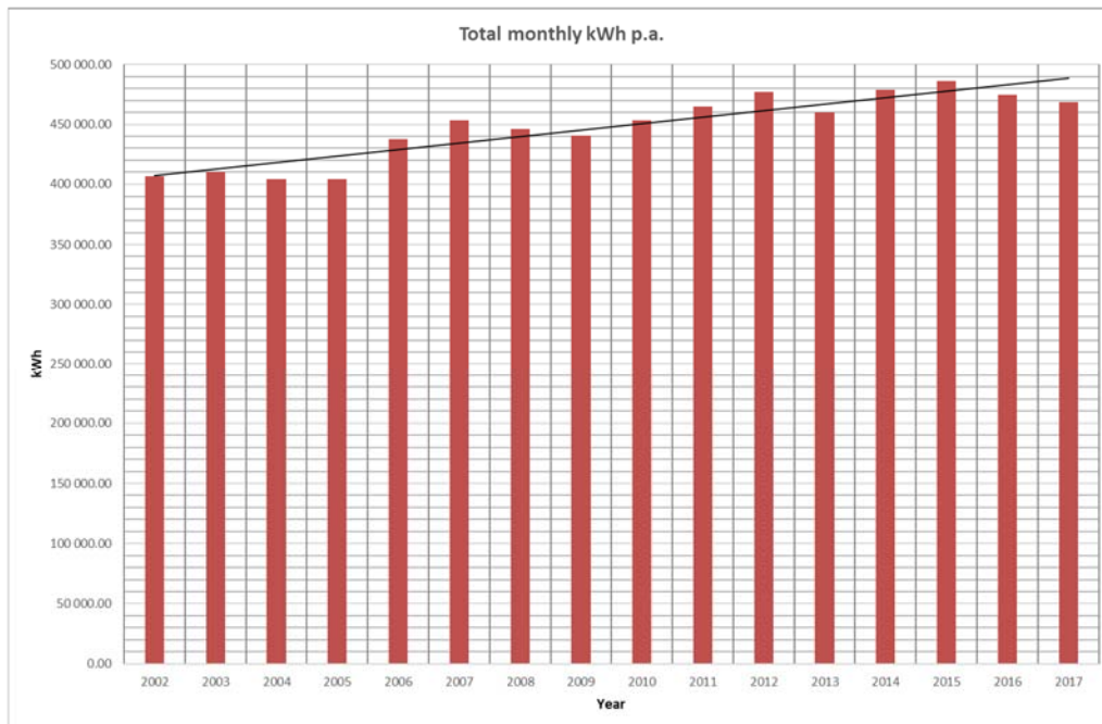
Figure 11: Actual recorded electrical energy usage for a 60 MVA NMD (Utility K)
