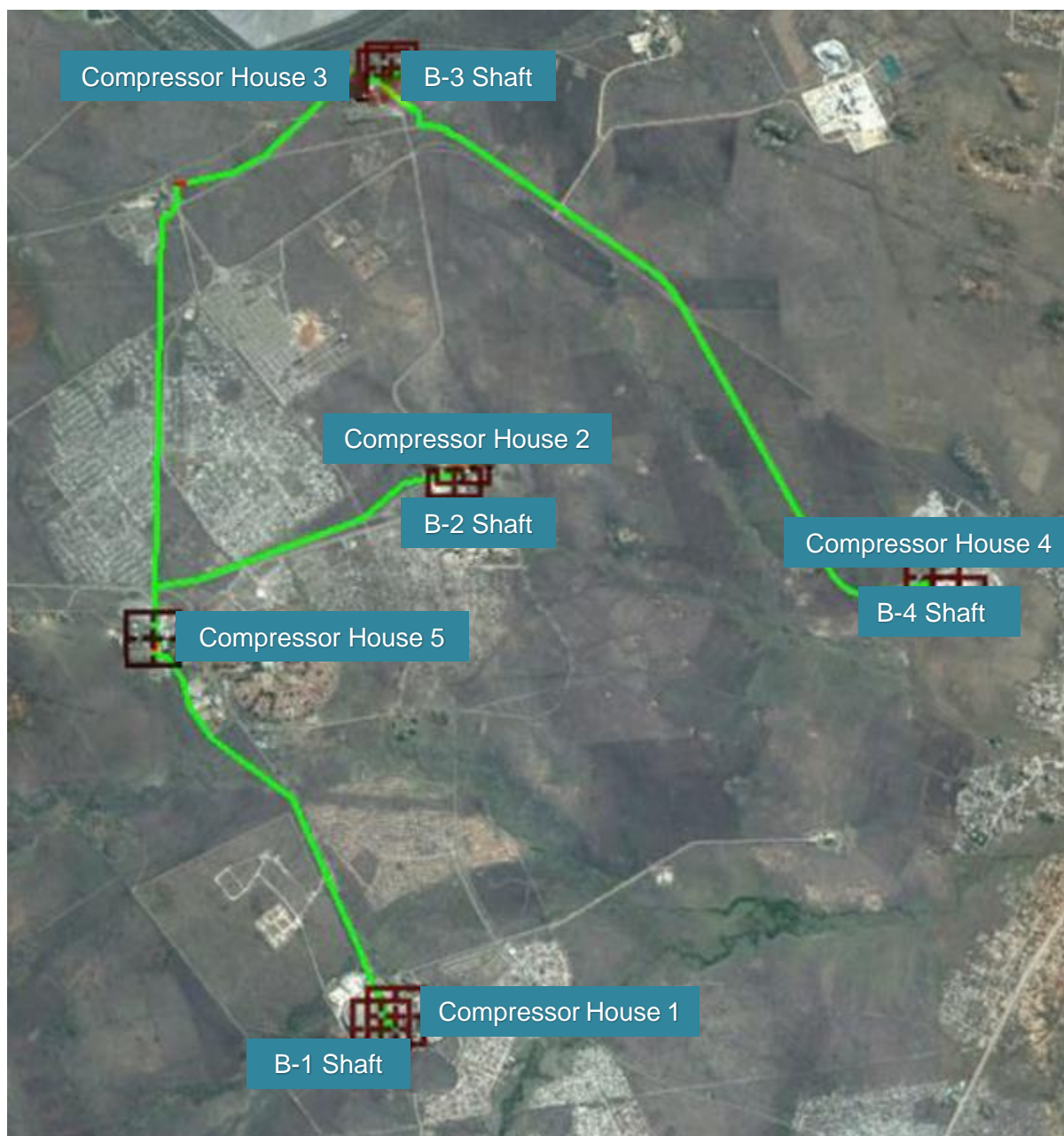
Figure 3-14: System B – satellite view of compressed air layout
