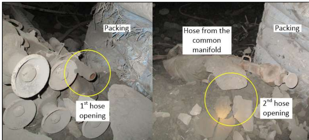
Figure 64: Photos of the open CA hoses 24-level UG2 West of Shaft E
