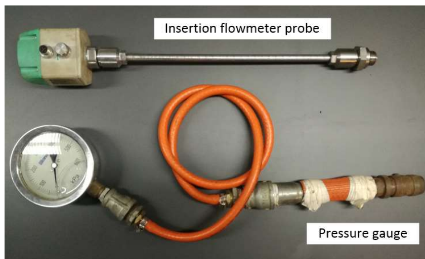
Figure 38: Portable compressed air measurement instrumentation
