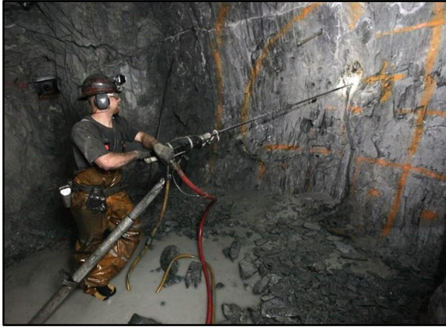
Figure 8: Mine worker operating a pneumatic drill [24]
