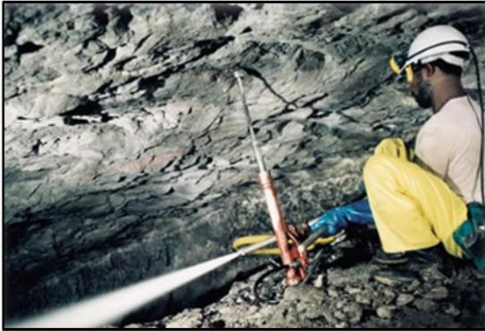
Figure 10: Mine worker operating a water cannon [26]
