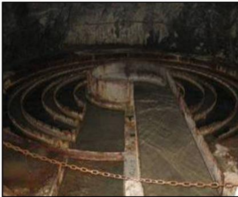
Figure 12: Mud settler used in a mine [26]
