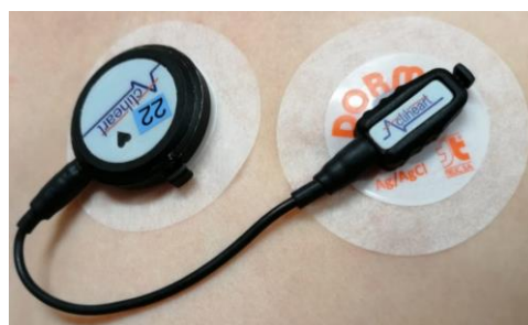
Figure 2: Fitting of the ActiHeart monitor to record heart rate, inter-beat-interval and physical activity.
