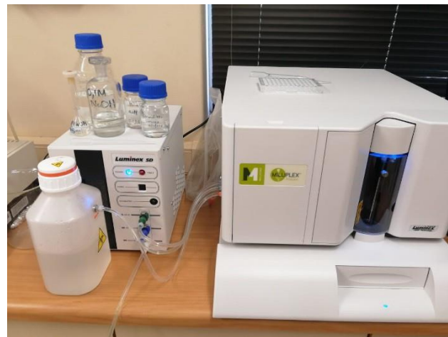
Figure 5: Luminex 200™ System - used to measure myeloperoxidase from serum samples.
