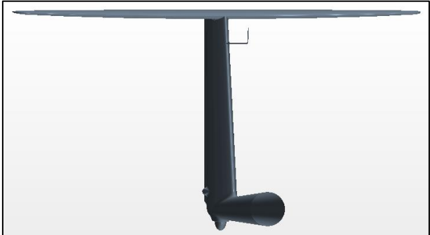
Figure 6-6: Pitch CFD model modified to simulate a 10° sideslip
