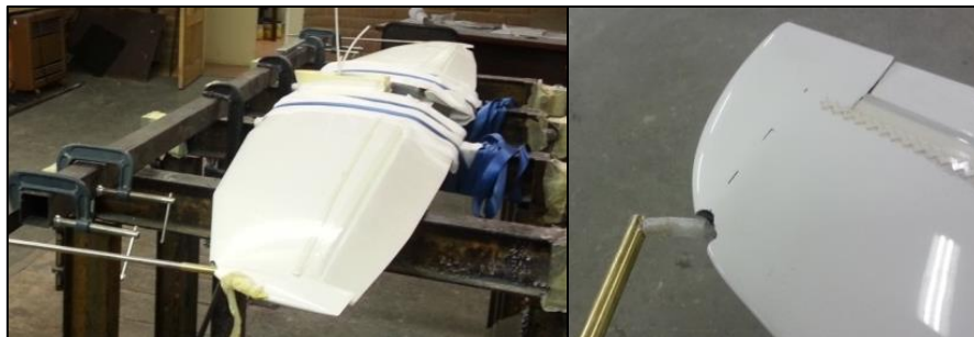
Figure 2-22: The total energy probe on the JS-1C moved to the tip of the horizontal tail plane (JS, 2014)
