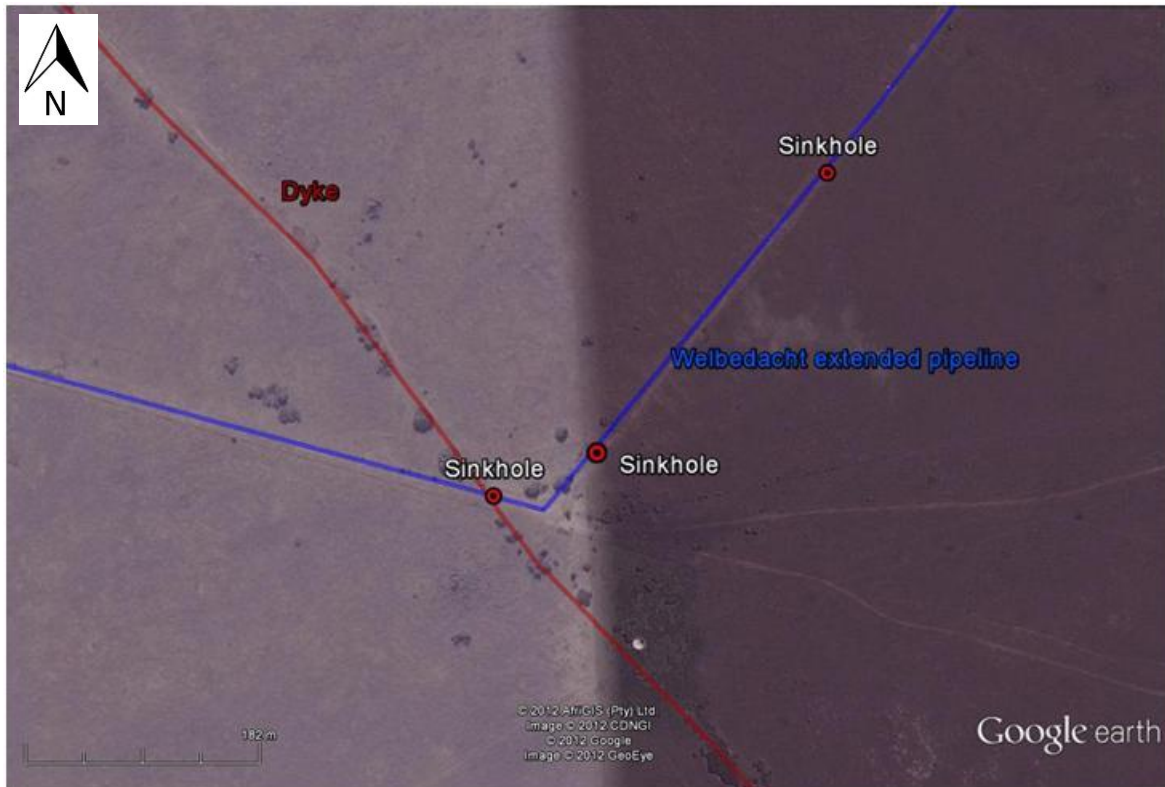
Figure 4-18: Google Earth graphic indicating sinkholes relative to pipeline
